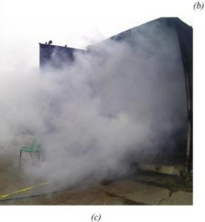
nail penetration at 50% SOC.a) was taken 26.47 s after the nail penetrated the module completely;b) was 35.47 s after penetrationc) 52.13 s after penetration.
