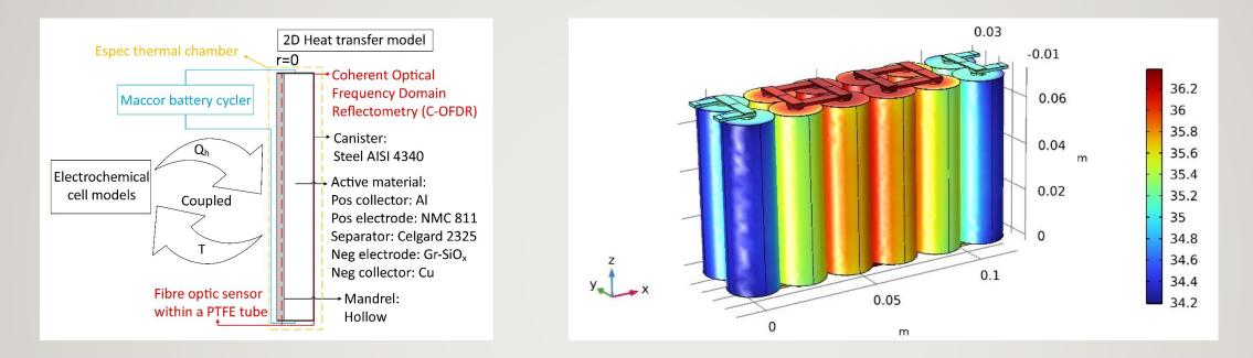
The electrochemical- thermal model (schematic view), in which the electrochemical models provide the cell thermal source to the thermal model (2D). The thermal model returns the obtained temperature to the electrochemical model. Validated with experiments
